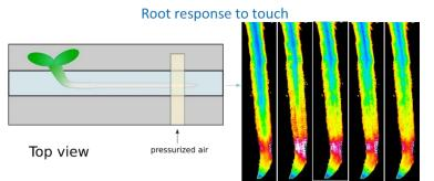
hydroponic chips for in-chip growth and microscopic study of *Arabidopsis thaliana* roots. We use microfluidic chips containing a pressure-driven PDMS microvalve in order to deliver a local mechanical stimulation to the root. Using genetically modified plant lines expressing fluorescent Ca<sup>2+</sup> nanosensors, we have revealed
